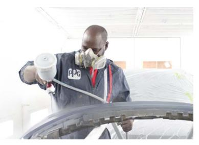
Spraypainting is a specialist skill; and Frans is a master - well versed in the art of selecting and adjusting the appropriate spraygun nozzles and applying different paint mixes and types, in order to get the proper paint flow and coating thickness.
